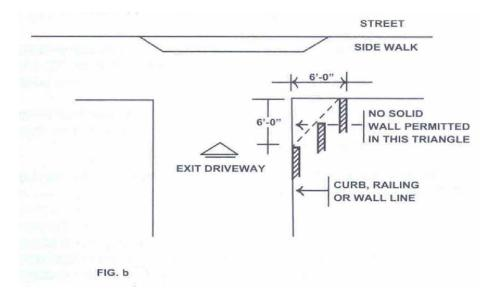
Fig-5.2 Chamfering at Driveway
